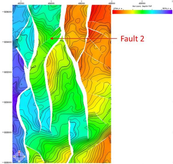
**Figure 9** (Left) Fault map of the Oseberg Syd area, on the Lower Tarbert horizon, showing the location of Fault 2 (as indicated by the red arrow)
