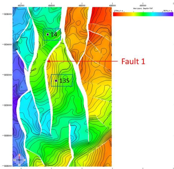
**Figure 3** Fault map of the Oseberg Syd area, on the Lower Tarbert horizon, showing the location of Fault 1 (indicated by the red arrow)
