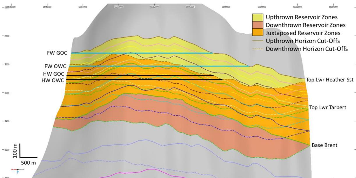
**Figure 4** Allan diagram (strike projection looking east) showing footwall intervals (solid colour) and hanging wall intervals (dashed). Yellow: footwall sands. Dark orange: hanging wall sands. Light orange: overlapping (juxtaposed) sands.
