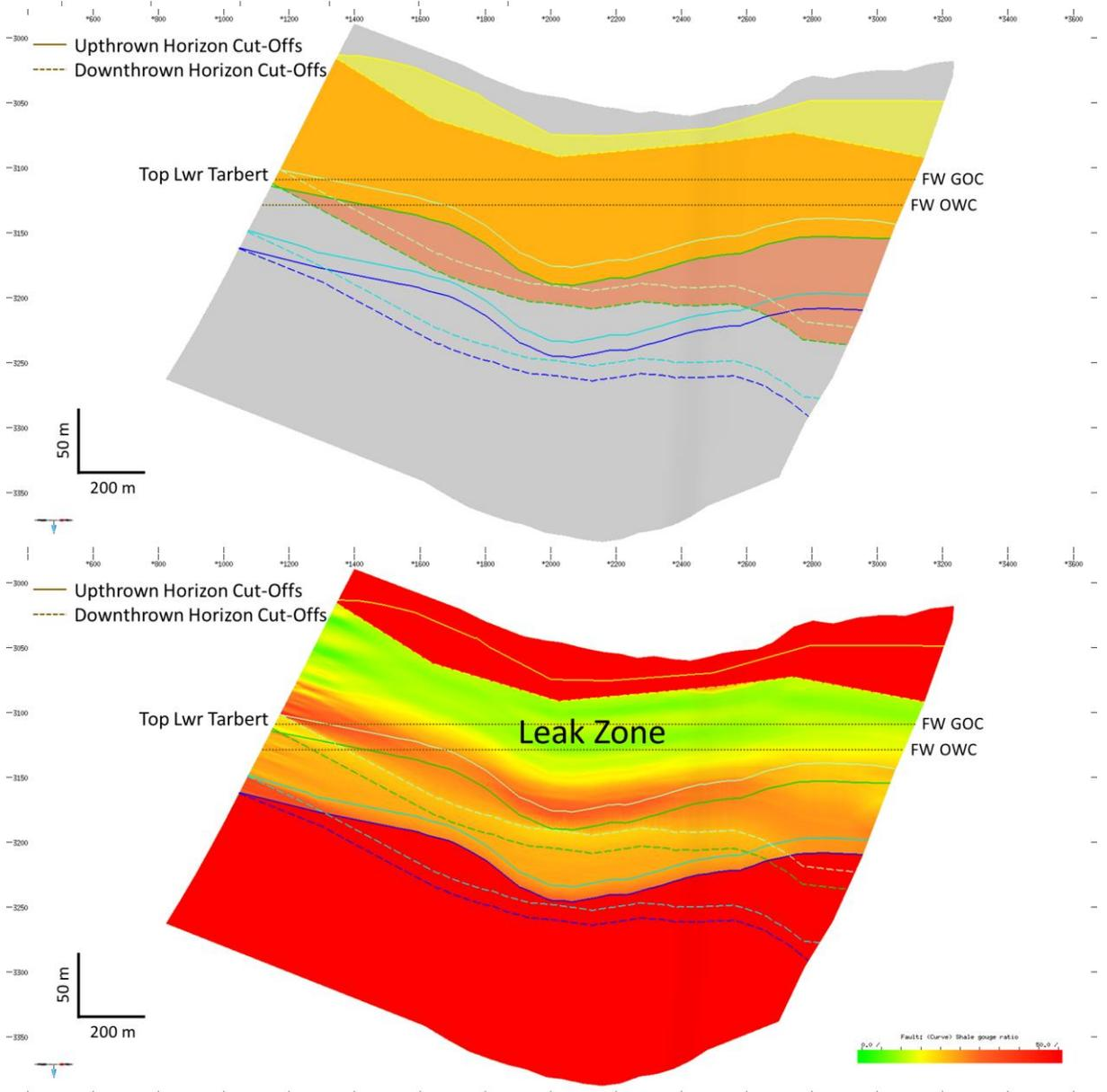
**Figure 10** (Below) Fault plane diagrams showing an Allan diagram (strike projection looking north) highlighting footwall horizon cut-offs (solid colour) and hanging wall horizon cut-offs (dashed). Yellow: footwall sands. Dark orange: hanging wall sands. Light orange: overlapping (juxtaposed) sands
