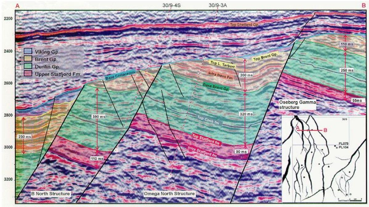
**Figure 2** E-W oriented seismic section through the north-western part of the area of study showing typical faulting and stratigraphy
