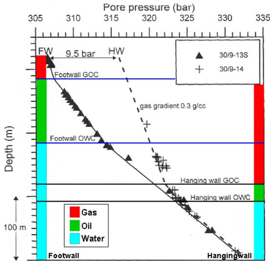
**Figure 6** Pressure profiles for Wells 13S (footwall) and 14 (hanging wall)
