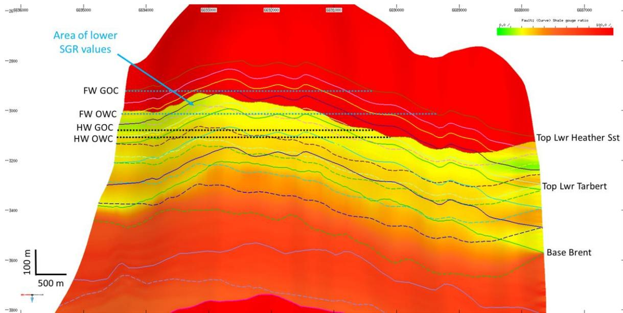
**Figure 5** Reservoir juxtaposition plot showing area of reservoir overlap colour filled with Shale Gouge Ratio. Low SGR values in pale yellow; high SGR values in red. Area of lower SGR values indicated by the blue arrow
