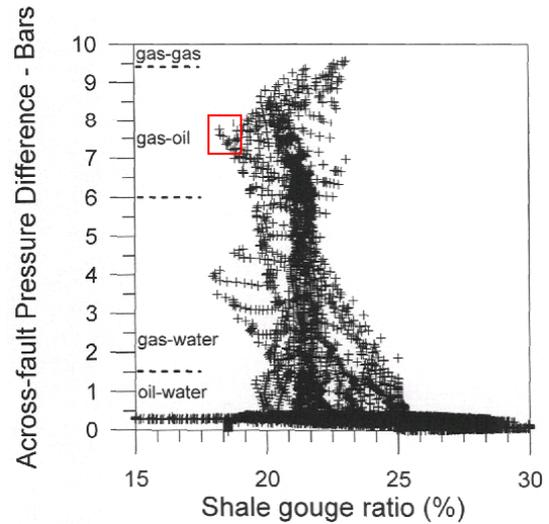
**Figure 7** Cross-plot of SGR versus across-fault pressure difference
